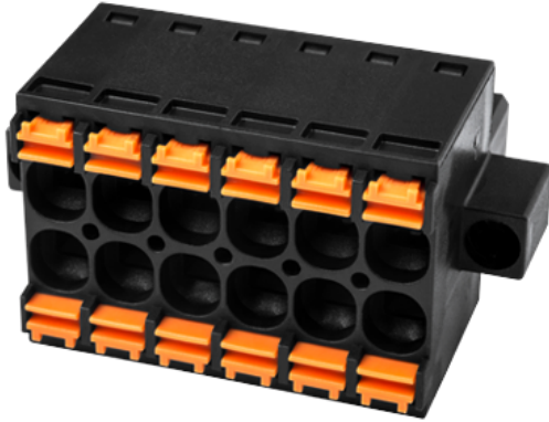
Twin connectors design, the pole number is half of the total connection points. photo shows a 12 connection product, the pole number is 06.
